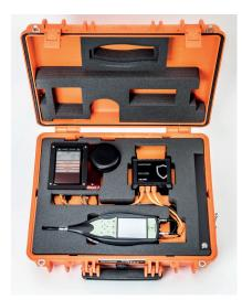
Portable noise monitoring is provided with portable unit Type NG-i359-PRT. This is functionally equivalent to the permanent version, but housed in a hand-carried waterproof case, suitable for monitoring periods of several months at a time. Also equipped with a 4G router, the portable unit communicates noise data in real time to Noise Guard server for storage and analysis.
