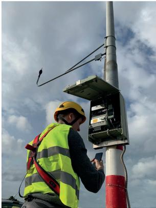
The retrofit is intended for existing Brüel&Kjær Type 3639 NMT users. The kit is a complete assembly which replaces all components inside the “green” cabinet with the new Noise Guard solution.
