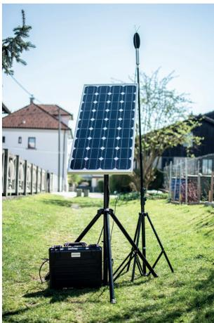
Running cables for power and communications to monitoring equipment around a construction site or industrial facility can be dangerous and unreliable. In suitable locations, stand-alone equipment may be provided, operating from solar panels and batteries. When coupled with mobile communications, this provides the best approach to ensure wire-free continuous monitoring around the site.
