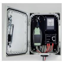
Noise measurements are based on our proven hardware, which continuously monitors noise at several locations around the world in a variety of applications including, industrial sites, ports, racetracks and construction sites.
