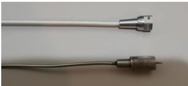
Figure 4. Examples of hardline cable terminations on the market, optimal cable on top, model 60016A, with Hex termination and complete fiberglass covering, rated at 1,000°F. At bottom, an underperforming hardline cable with knurled termination, no fiberglass coverage, and lower temperature rating of 900°F.
